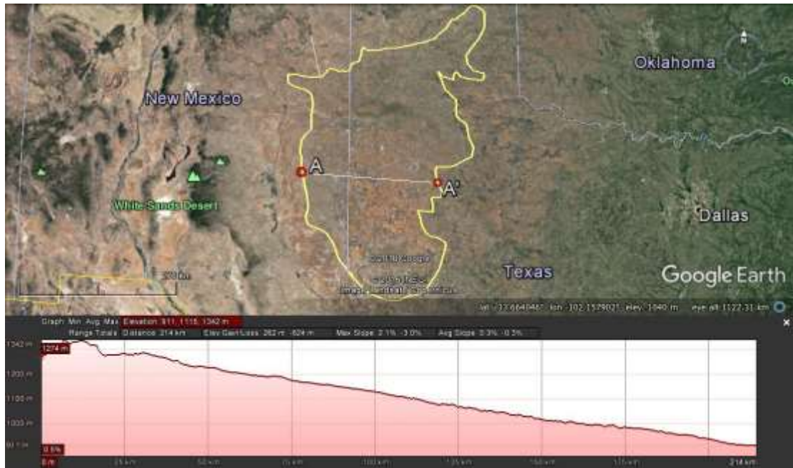
Figure 1.1. Topographic profile of the modern SHP surface. SHP is outlined in yellow. The profile runs W-E, in accordance with modern drainage patterns. Dimensionless slope of this surface = 0.0020. Vertical exaggeration of profile = ~500X. Map data ©2016 Google.
