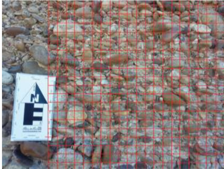
Figure 3.7. Example of digital grain size analysis. Taken from Field Site B, Location 3. A 2-cm grid was overlain on outcrop images, and grain diameters were measured at grid intersections. An intersection falling on a grain less than 1 cm in diameter was counted as matrix.
