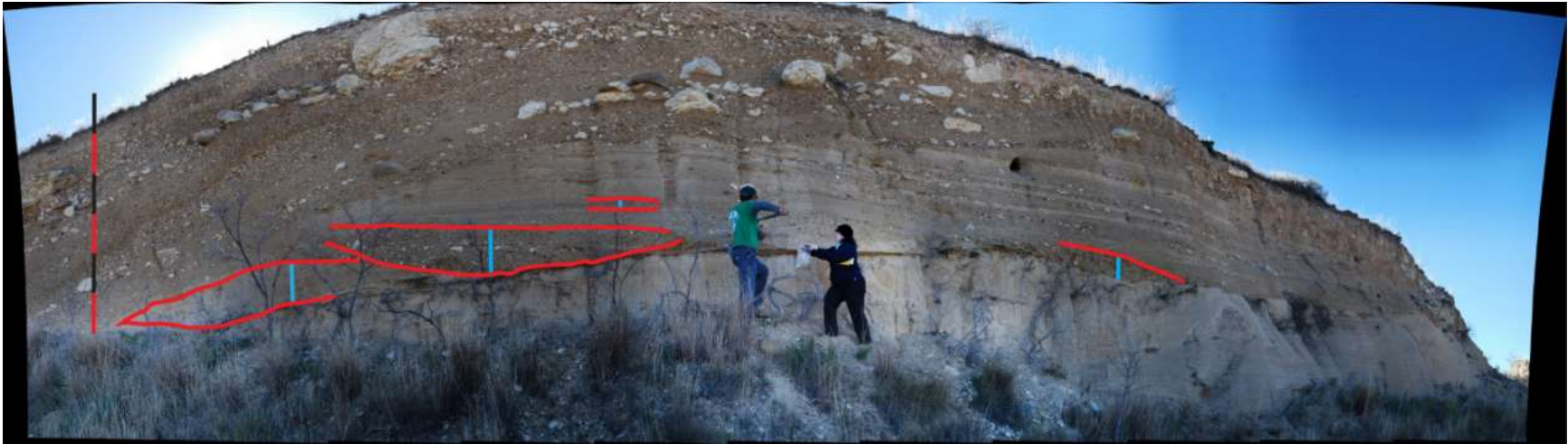
Figure 3.8. Digital bedform measurement. Image of Field Site B, Location 2, showing digital measurements for bedform heights. Scale bar = 3 m.
