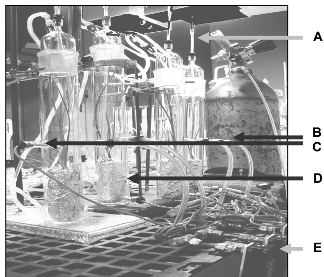
Figure 1: Individual Growth Chambers (interior dimension 45 cm tall x 7 cm diameter) with onion seedlings: port with syringe for exchanging the nutrient media [A], port with absorbent filter for volatile organic collections [B], port with sensor for temperature/moisture measurements [C], nutrient media pack wrapped in aluminum foil [D], and flow meters for measuring the air pulled from the chamber [E].
