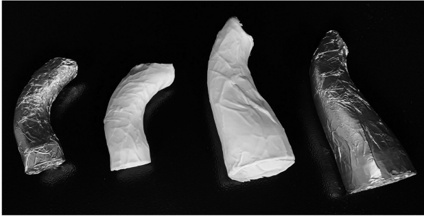
Fig. 13. 3D printed mandrels and AutoOpt TEVG for Case 1 and Case 2.
