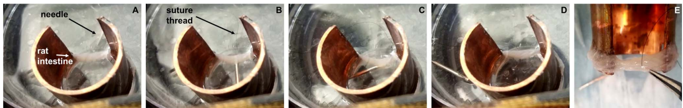
Fig. 12. NdFeB needle with thread is guided towards suspended rat intestine (A) and pulled through rat intestine (B). Further manipulation pulls suture thread through intestine (C, D), with (E) showing closeup of thread through intestine.
