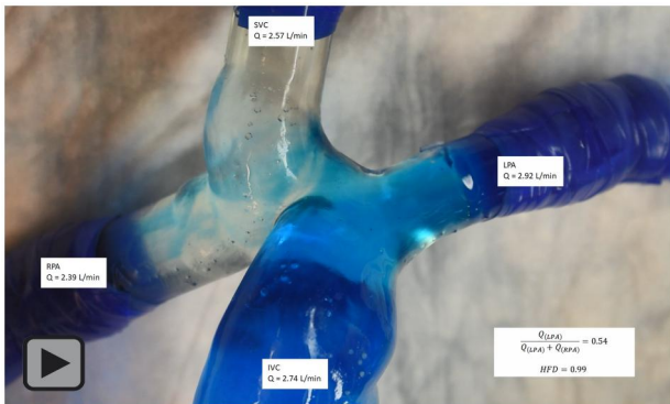
Video 2: Visualization of the tracer dye in a clear CCPC.
